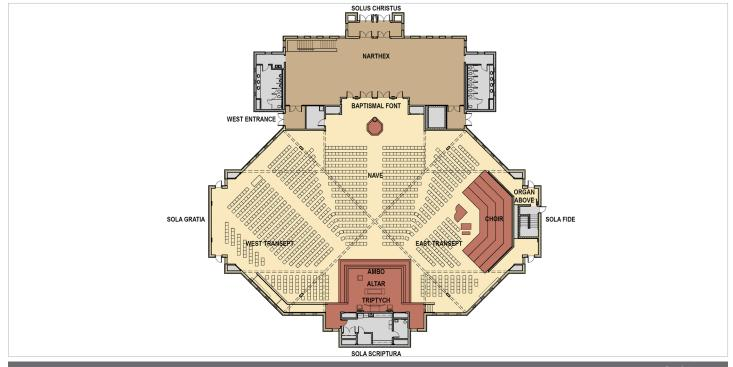
The more these forms can be translated between interior and exterior, the stronger the design. Here at The Chapel of the Christ, we designed massive wood arches and beams to define the volume. The arches span one hundred feet to intersect in the middle of the worship space, carrying the beams that establish the nave and the transept. This form-giving structure
